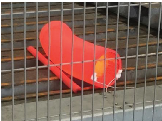
Bend during heat treatment
